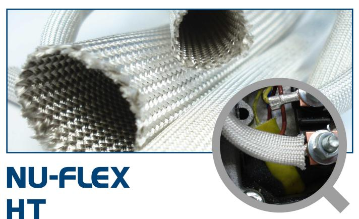
NU-FLEX HT is a tightly woven, flexible, continuous filament electrical grade 100% fiberglass braid that is heat treated to remove all organic matter and then saturated with an acrylic binder.
